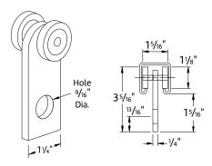
Use With AS 200. Stainless Steel Ball Bearings \*Based on standard dimensions for channel Std Pkg: 20 · Wt/100 pcs: 46 lbs.
