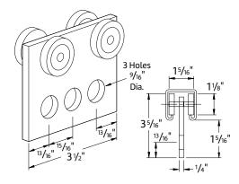
Use With AS 200. Stainless Steel Ball Bearings \*Based on standard dimensions for channel Std Pkg: 10 · Wt/100 pcs: 110 lbs.
